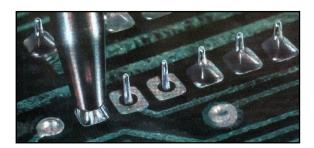
The Vacuum Desoldering Tool utilizes a tubular tip which transmits heat to an individual solder joint and vacuum removes solder, leaving leads and holes clean.
